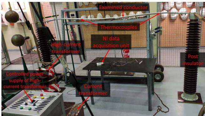
Fig. 1. Measurement arrangement
