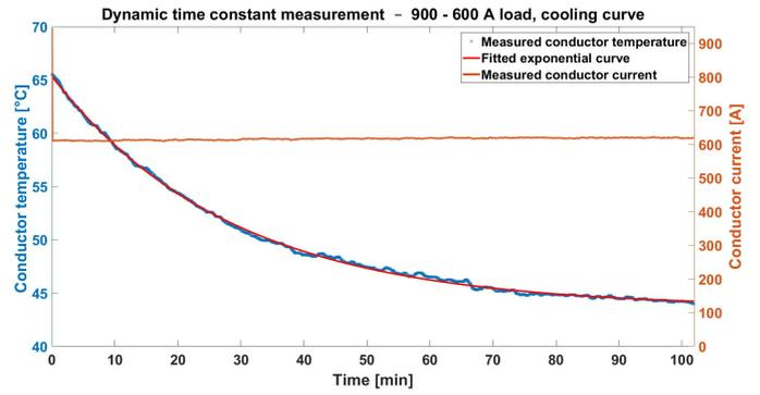
Fig. 4. Thermal time constant measurement with dynamic method – cooling curve
