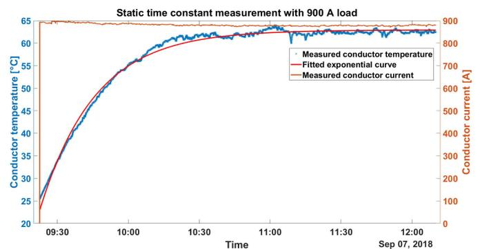
Fig. 2. Thermal time constant measurement with 900 A load
