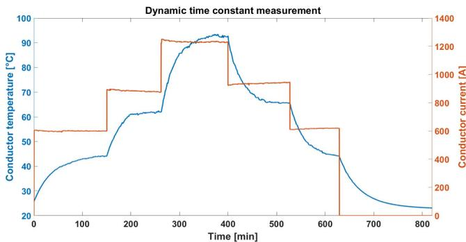
Fig. 3. Thermal time constant measurement with dynamic method
