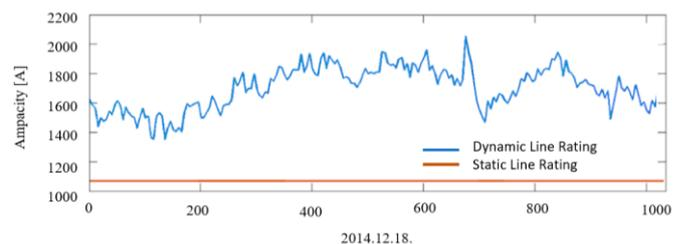
Fig. 5. Comparison of ampacity in case of SLR and DLR [12]
