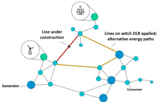
Fig. 6. Illustration of the use of DLR if LW cannot be applied on the line [13]
