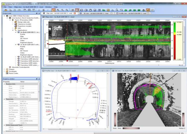
**Figure 3:** Typical results of profile measurements as 3D, 2D unwound plane and 2D profile view
